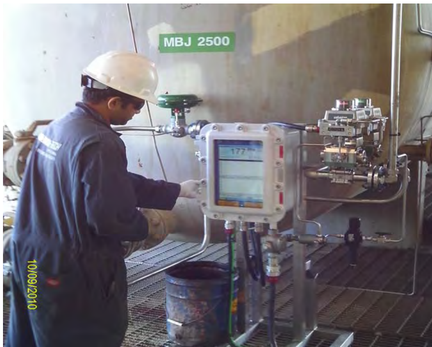
Figure 12: O&G Concentration of 177 PPM at the Skimmer Outlet.
